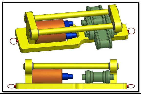
WARNING: Always wear safety glasses, gloves, and other protective clothing when using chain press. Due to the nature of pressing operations, metal chips can break off during pressing operation if not aligned correctly. The Cincinnati Mine Machinery Co. will not be held responsible for any injuries caused during the use of the chain press. Pin alignment is critical for your safety and the safety of your co-workers.
